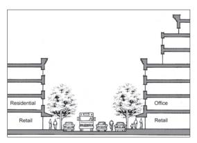
Figure 3.C.74: Taller buildings should be designed to step back or modulated in order to create compatible building forms on either side of a street.
