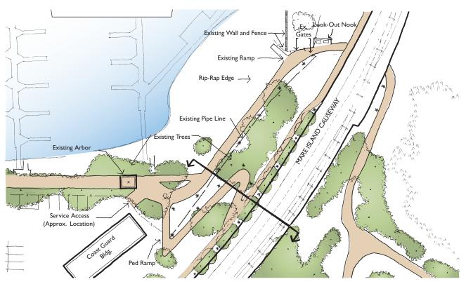
Figure 3.D.49: Sketch Concept of Trail Connection under the Causeway Overpass (arrows and lines indicate location of section - See Figure 3.D.50)
