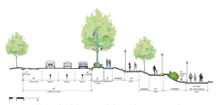
Figure 3.D.50: Partial Cross Section of Mare Island Causeway at Proposed Multi-purpose Trail Ramp Connection to Promenade Extension
