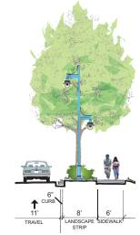
Figure 3.D.42: Partial Cross Section of Typical Sidewalk and Lighting Improvements on Southside of Mare Island Causeway (1)
