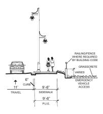
Figure 3.D.43: Mare Island Causeway (Constrained) - Partial Cross Section (2)
