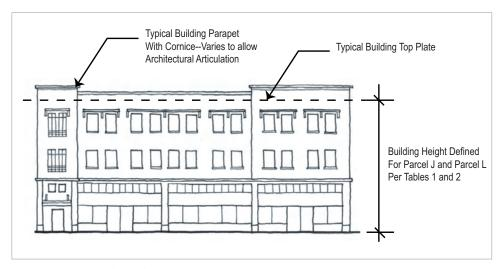
Figure G: Prototypical Top Plate Location
