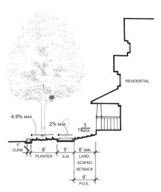
Figure 3.D.30: (Option A - Preferred) Harbor Way Partial Cross Section at Parking with Tree Lawn and Separated Sidewalk
