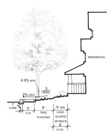
Figure 3.D.31: (Option B)Harbor Way Partial Cross Section at Parking with Monolithic Sidewalk 1
