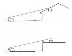
Figure 3.A.46: Mechanical equipment can be accommodated within rooflines or behind parapets.
