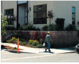
Figure 3.C.69: (Example of Poor Design) Planters should not exceed a comfortable pedestrian-scaled height. These are too tall.
