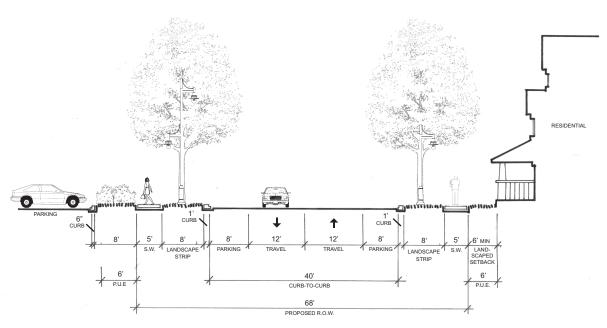
Figure 3.D.32: Harbor Way Partial Cross Section at Parking
