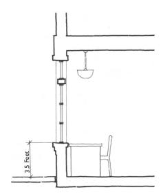
Figure 3.A.34: Keeping window sills at 3 feet 6 inches of the finish floor allows desks to be placed against window walls.
